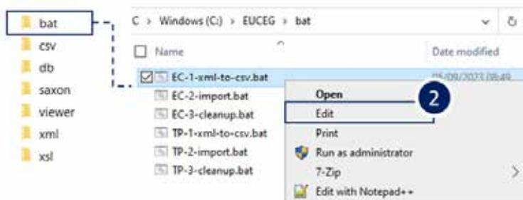
In the <bat> subfolder, right click on the EC-1-xml-to-csv.bat (resp. TP-1-xml-to-csv.bat) and select edit (or drag and drop the BAT file into a Notepad++ window).
